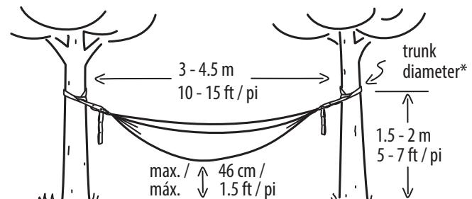
\* wrap the strap around a tree with a trunk diameter of at least 30 cm / 12 inches for stability.
