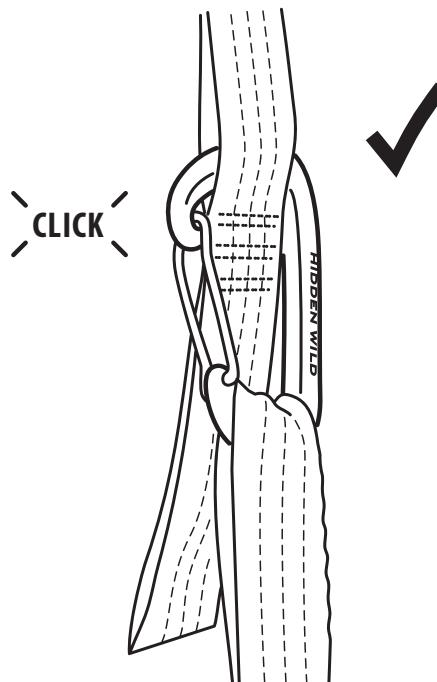
**!** Straps must be flat and straight. Gate must be touching the nose and close the loop.
